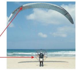
When the hands are near the body only the tips are pulled down. Is intended primarily for accelerated maneuvering.
