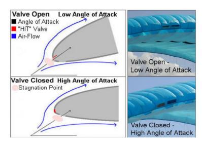
The F3 is equipped with an Active HIT Valve system (patent pending) to improve the overall performance and safety of the wing especially during accelerated flight.
