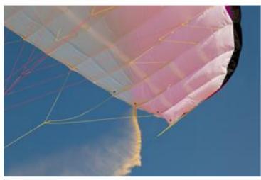
The F3 is equipped with Butt-hole II, which automatically clears smaller particles such as sand, grass and stones from the wing.
