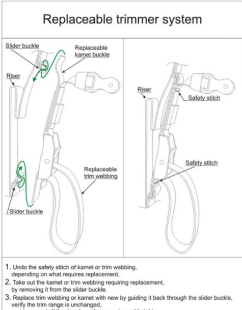
on trim speed all the riser branches are at equal height. When kamet fully released it should not retain any load (all the load is on the fully released D branch of the riser).
