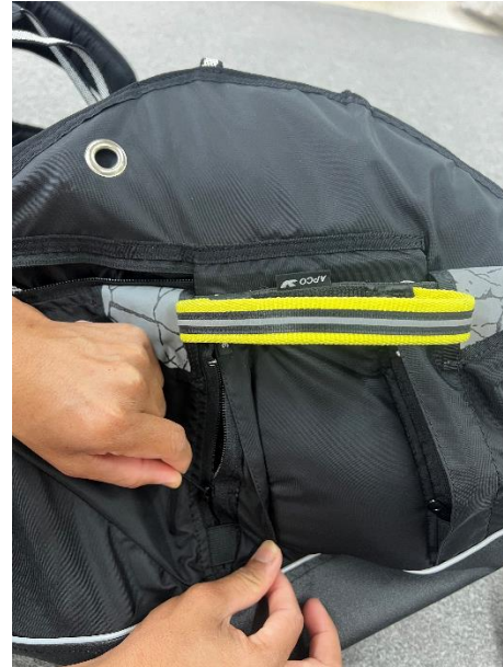
Close the two reserve container zips by running the sliders up to the locking loops (all the way).
