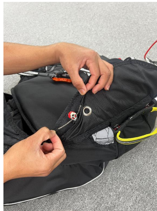
Pass the line through the pulley and then follow through the eyelet.
