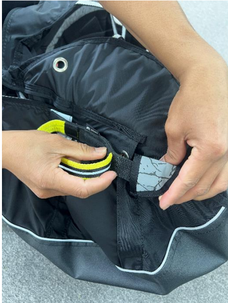
Stow the cable ends and reserve handle ends in the gray sleeves.
